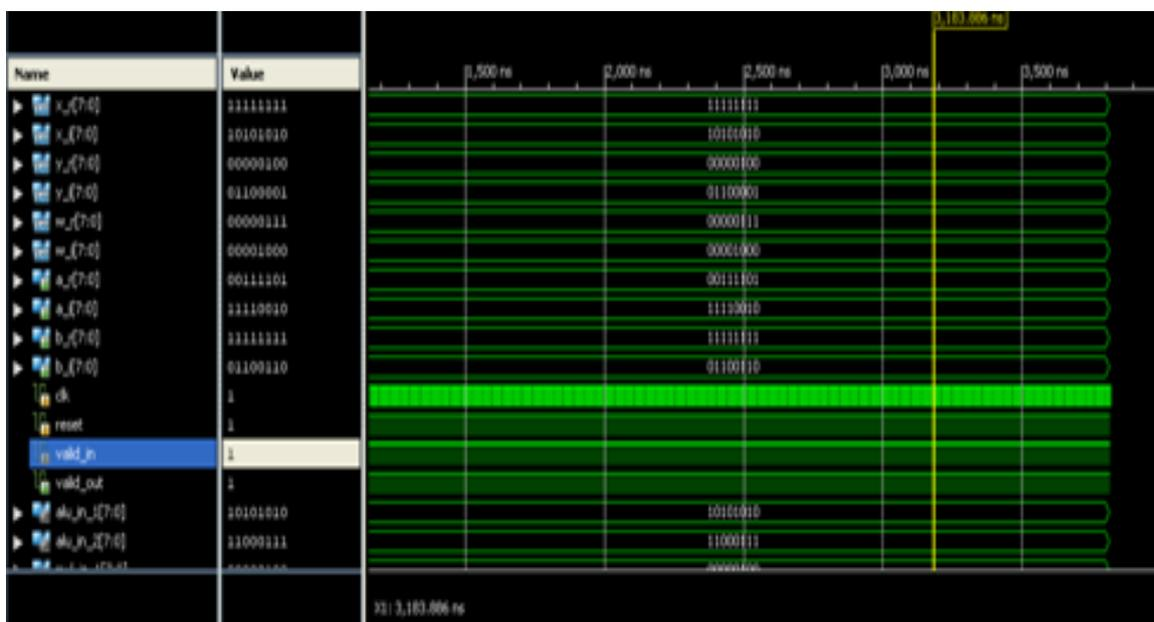
Figure 5: simulation waveform of 8-pt FFT using ALU
