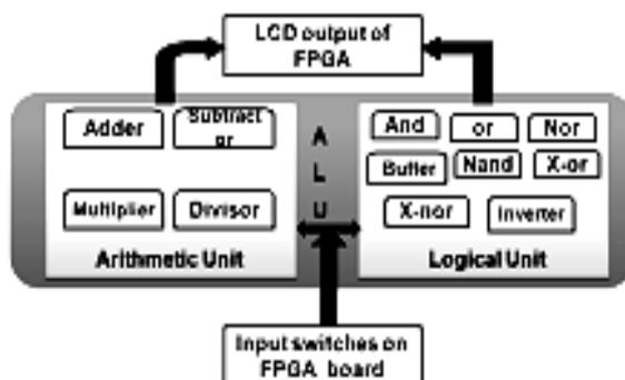
Figure 2: Block Diagram of ALU
