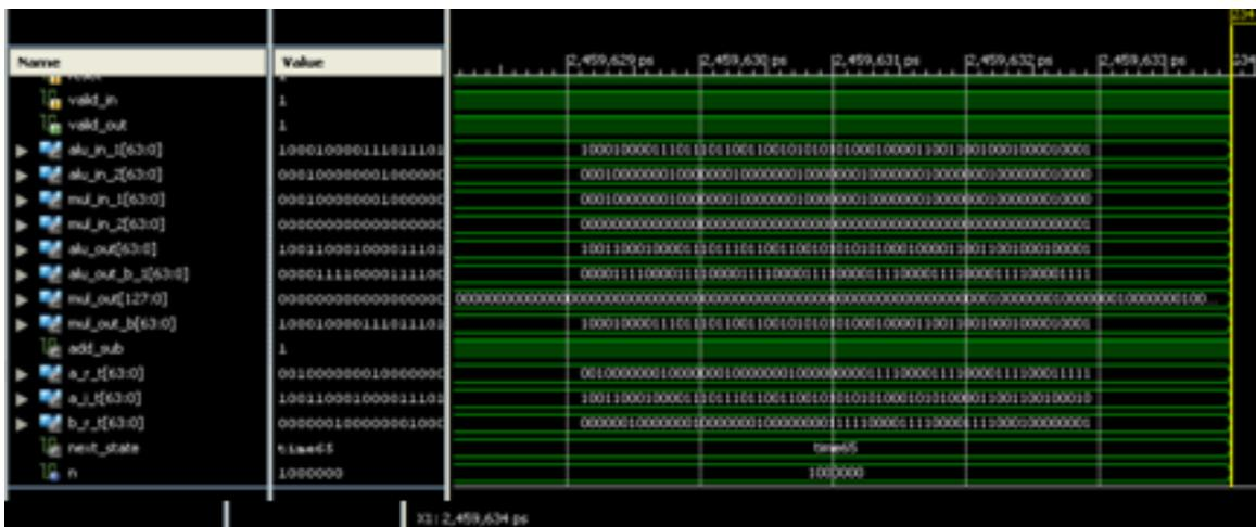
Figure 7: simulation waveform of 64-pt FFT using ALU
